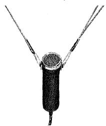
Figure 10-8. A typical lavalier microphone
